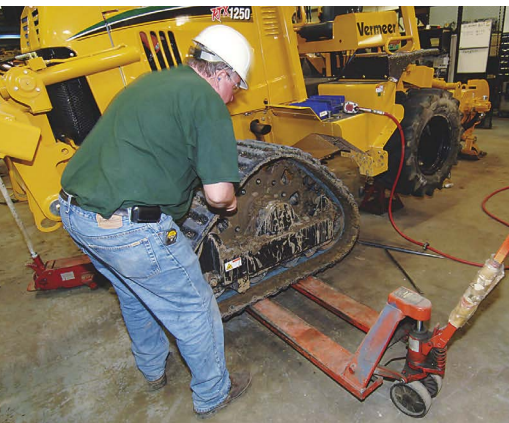
According to Vermeer, switching between the rubber quad-track undercarriage and the wheeled undercarriage takes two technicians about 2.5 hours.
