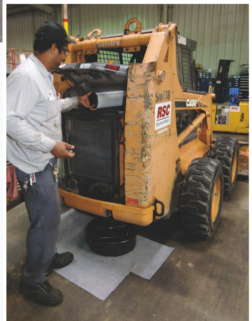
RSC East Chicago mechanics use absorbent oil pads to catch spills, toss them in a marked can in each work bay, and dispose of them with waste oil.
