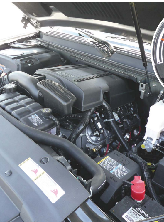
A hefty 6-liter 332-horsepower Vortec V-8 acts as a V-4 whenever possible and shuts down frequently in stop-and-go driving. The hybrid's electric system, partly housed in the far corner of the engine compartment, operates at 300 volts.
