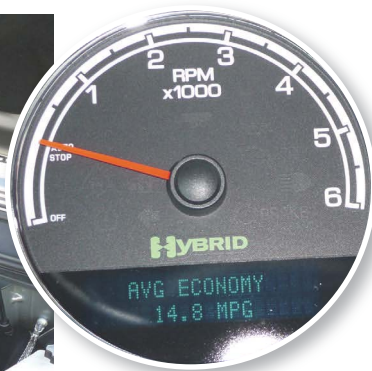
Tach needle rests on Auto Stop as the engine naps at a red light; it restarts instantly when needed. Readout shows unimpressive economy during heavy-footed demonstrations, but the hybrid's supposed to get 20 to 21 mpg in town.
