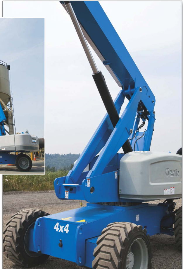
Virtual pivot assembly (above) keeps boom weight over the chassis' center of gravity. Single-cylinder boom design (inset) reduces boom weight and lowers service and repair costs.
