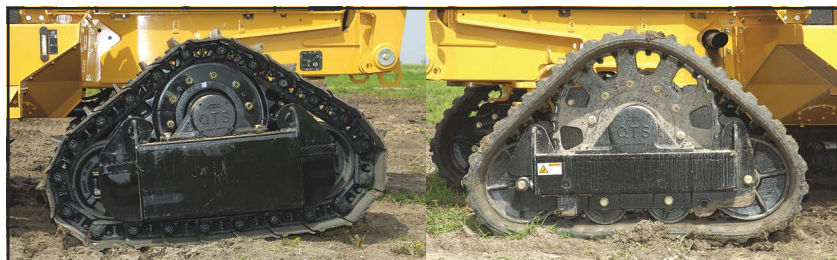
Steel tracks (left) are designed like crawler-dozer undercarriages. Once installed, the steel-track modules become a permanent undercarriage. The rubber-track modules (right) spread the tractor's weight across the belt via a system of wheels.
